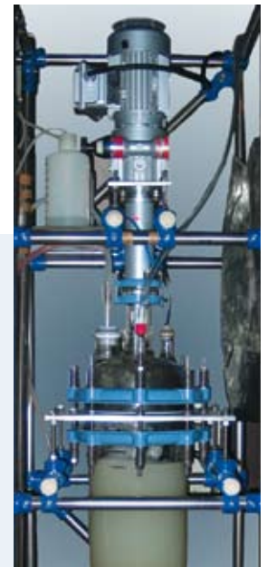
▲ Reactor for the biological production of hydrogen.
